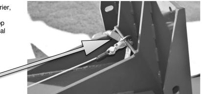
**STEP 5** You may now remove the barriers using the hauler jack or manual tow bar (See *Archer 1200 Deployment Instructions.pdf*). Use the attached winch cable to support movement down the ramp. Remove winch cable when barrier is on a vertical surface.
