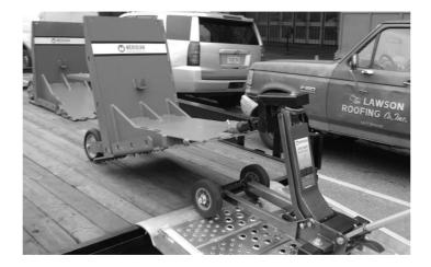
**STEP 6** After barrier deployment, secure all accessories (hauler, tow bar, cables) in the back of the trailer with tie downs. Replace the ramp in the side slot and secure with wing nuts. Replace rear trailer gate rails.
